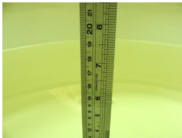
Fig 6.2 Photo of Liquid Height for Body SAR
