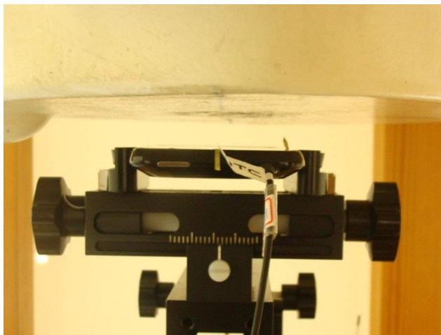
Front of the DUT with Phantom 1 cm Gap for DUT with Earphone 2
