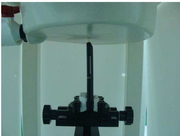
Top Side of the DUT with Phantom 1 cm Gap for DUT without Earphone
