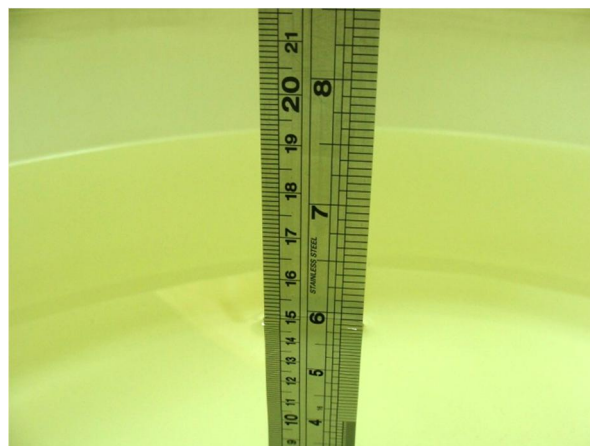
Fig 6.2 Photo of Liquid Height for Body SAR
