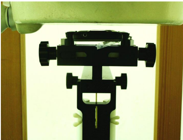
Rear Face of the DUT with Phantom 1.0 cm Gap for DUT without Earphone
