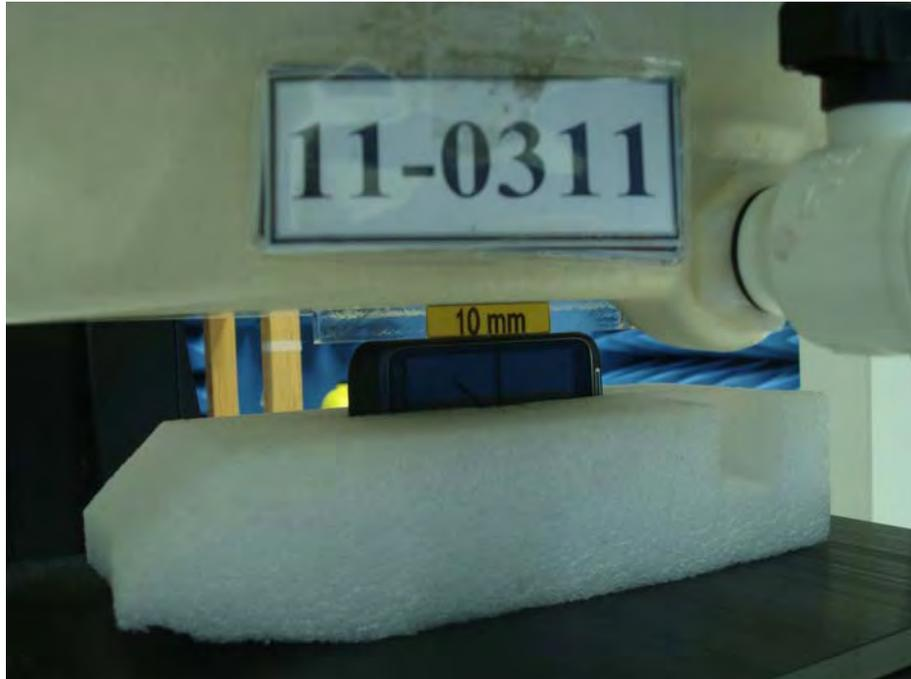
Figure 9. Body SAR Test Setup (Flat Section)
