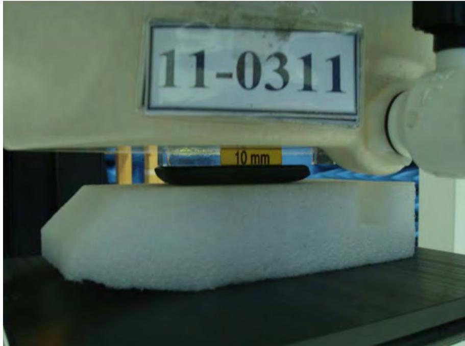
Figure 6. Body SAR Test Setup (Flat Section)
