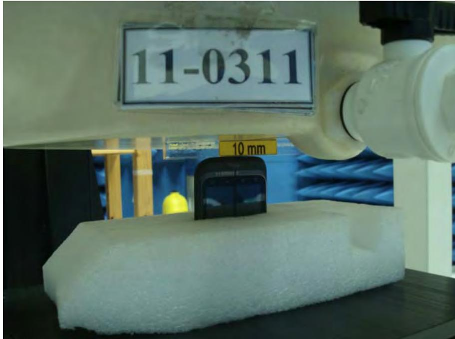
Figure 11. Body SAR Test Setup (Flat Section)
