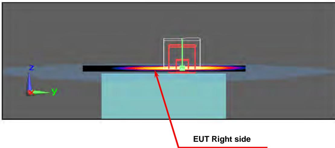
Body Setup \_ Edge Bottom to Phantom 10mm
