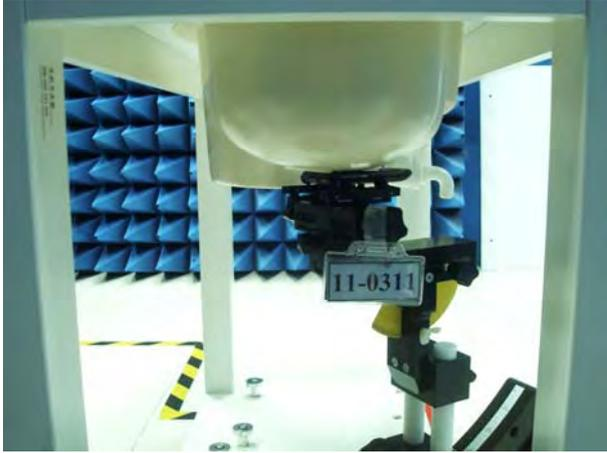
Figure 1. Right Head SAR Test Setup (Cheek)
