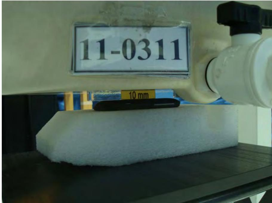
Figure 8. Body SAR Test Setup (Flat Section)
