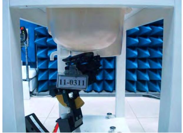
**Figure 4. Left Head SAR Test Setup (Tilted)**
