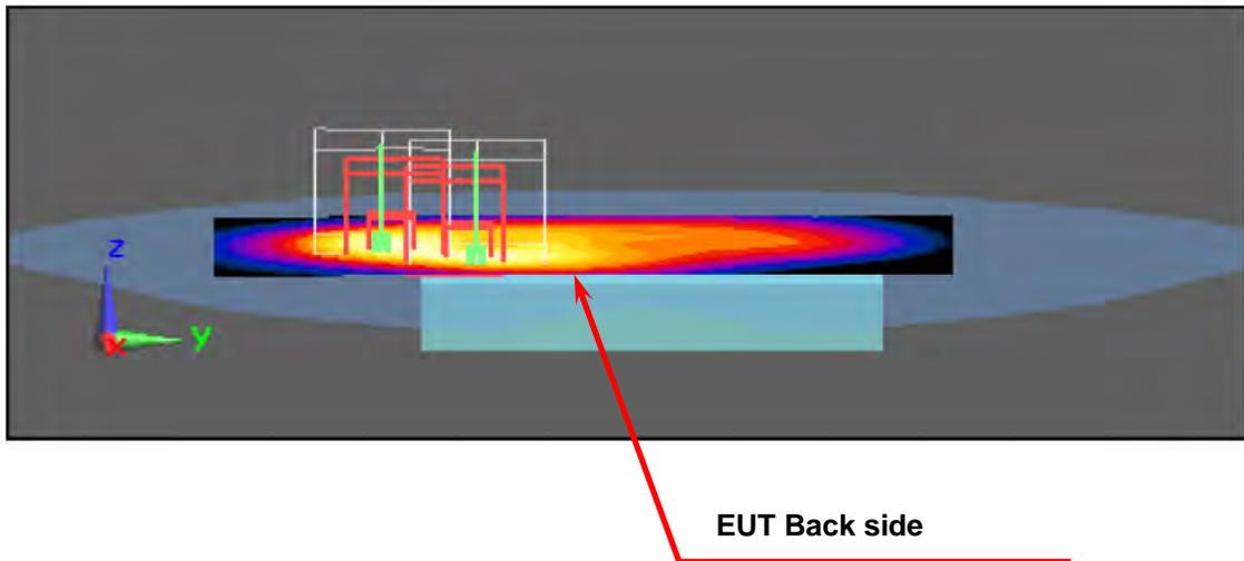
Body Setup \_Back Surface to Phantom 10mm
