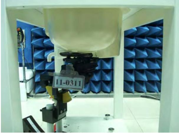
**Figure 3. Left Head SAR Test Setup (Cheek)**
