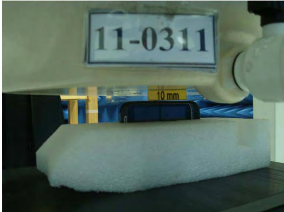
Figure 10. Body SAR Test Setup (Flat Section)
