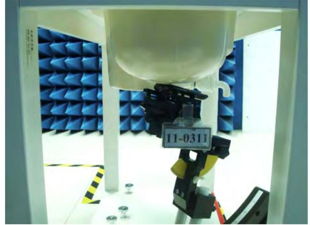
Figure 2. Right Head SAR Test Setup (Tilted)
