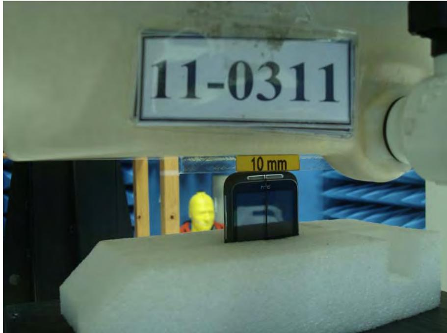
Figure 12. Body SAR Test Setup (Flat Section)
