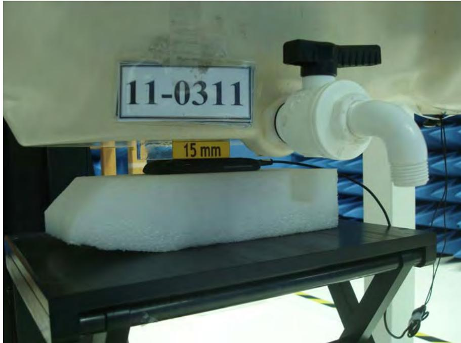
**Figure 7. Body SAR Test Setup (Flat Section)**
