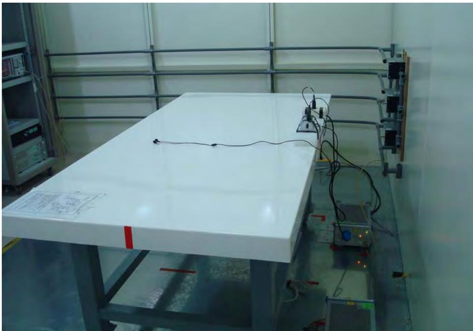
**Radiated Emissions Test Configuration:**
