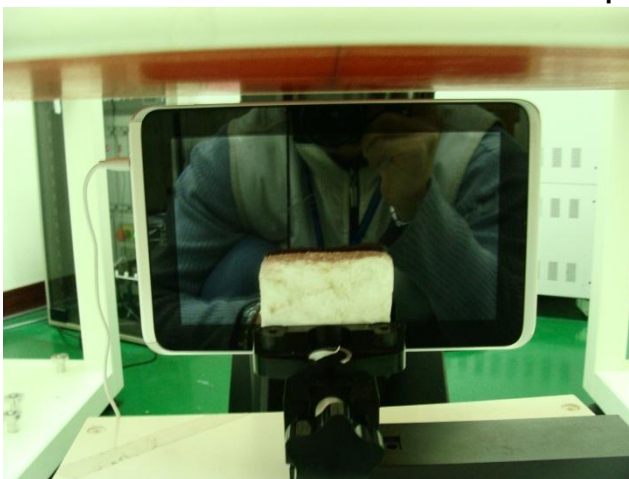
Right Side of the DUT with Phantom 0.5 cm Gap
