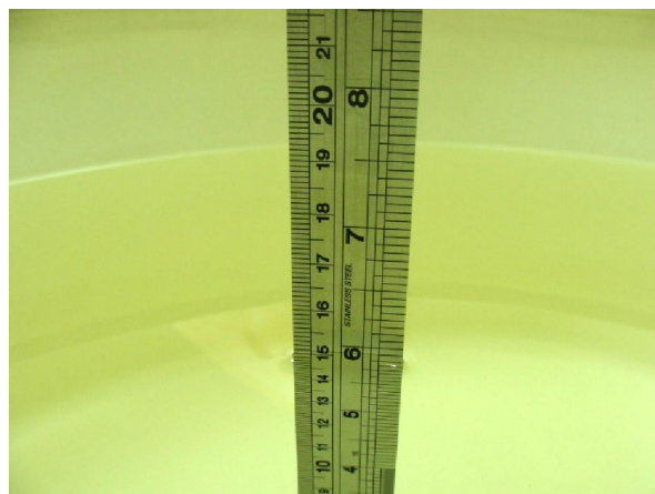
Fig 6.2 Photo of Liquid Height for Body SAR
