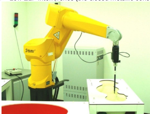
Fig 5.5 Photo of DASY4
