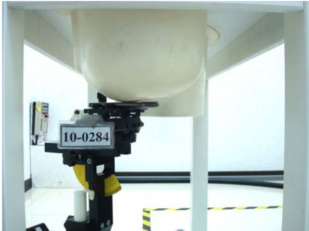
Left Head SAR Test Setup (Cheek)
