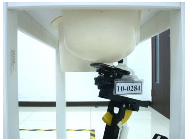
Right Head SAR Test Setup (Tilted)
