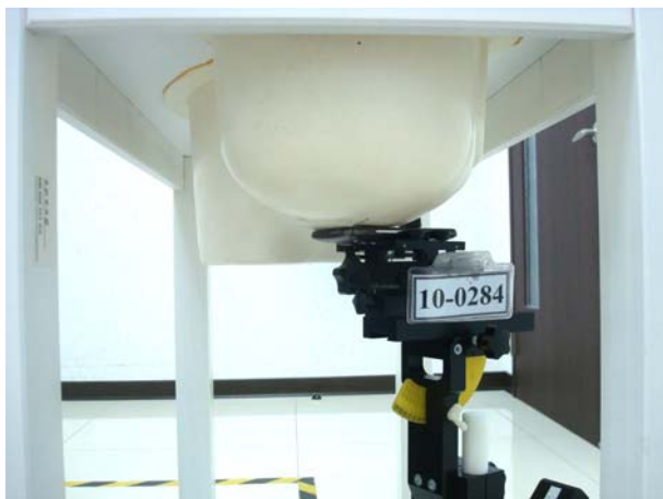
Right Head SAR Test Setup (Cheek)
