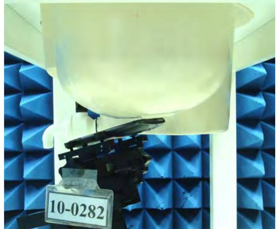
**Figure 4. Left Head SAR Test Setup (Tilted)**
