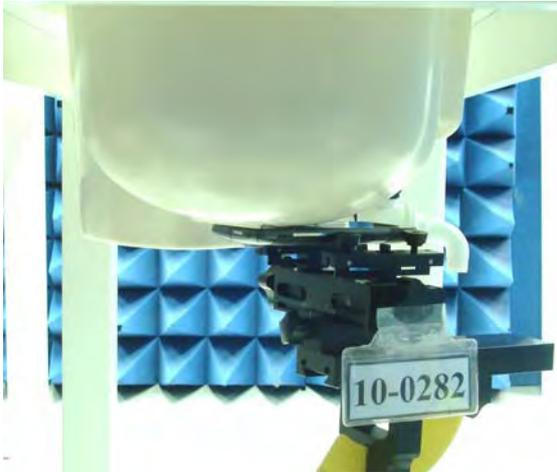
Figure 1. Right Head SAR Test Setup (Cheek)
