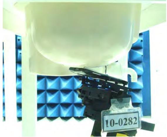
Figure 2. Right Head SAR Test Setup (Tilted)
