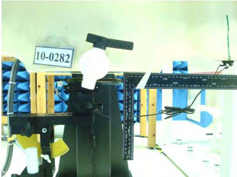
**Figure 5. Body SAR Test Setup (Flat Section)**
