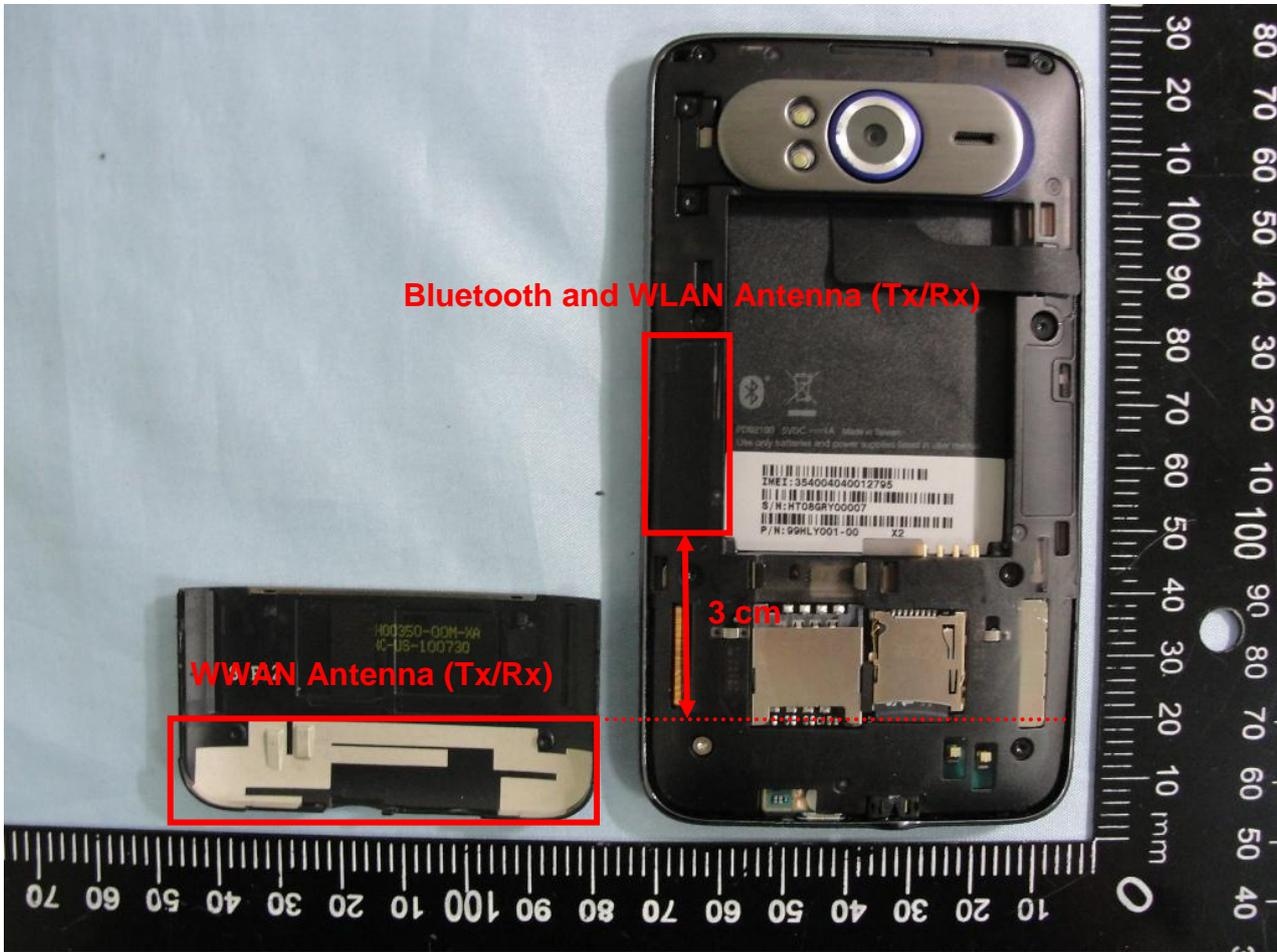
Bluetooth and WLAN Antenna (Tx/Rx)
