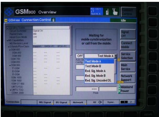
d: GPRS Multi Class10: support maximum uplink=2, since to enable 2 uplink slot and setting the power on Gamma 3(33dBm)
