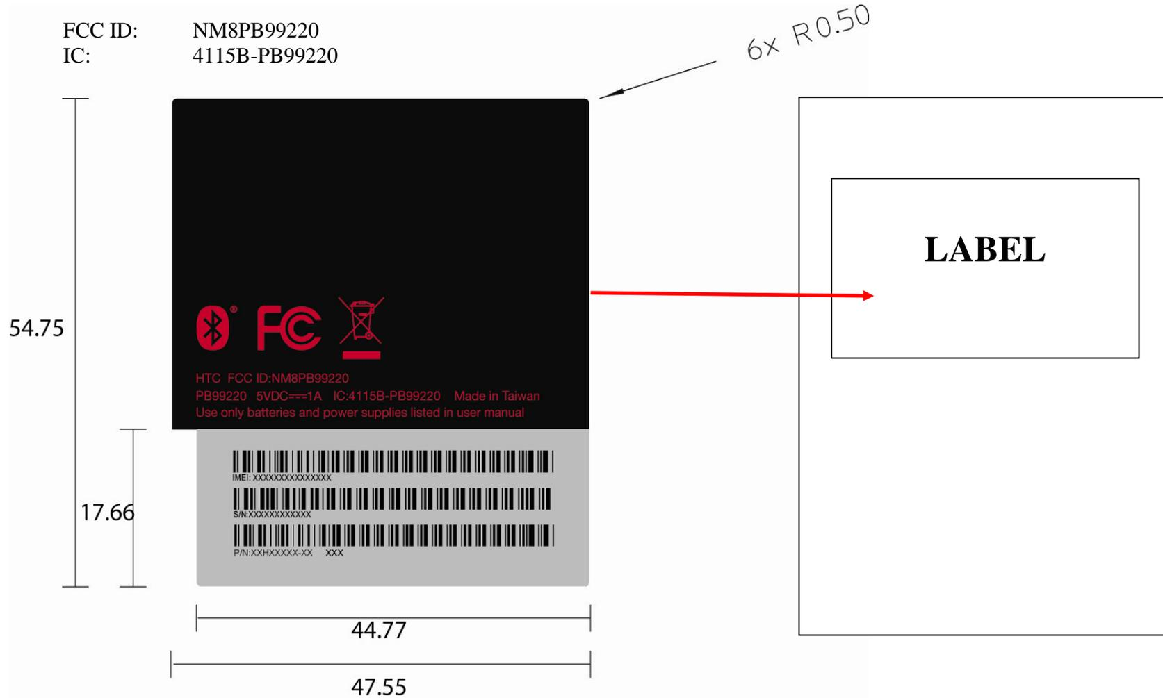
NOTE: label on internal PCB board, not on back cover
