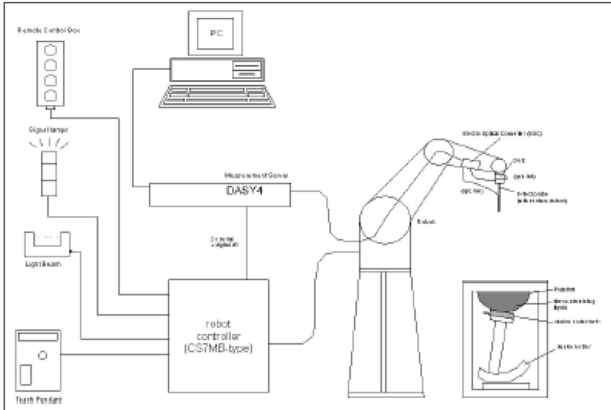
**The DASYS4 system for performing compliance tests consists of the following items:**
