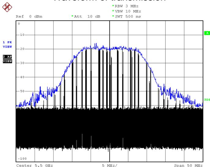
3) Radar signal 1 is applied to the Master device and WiFi traffic signal stop immediately.
