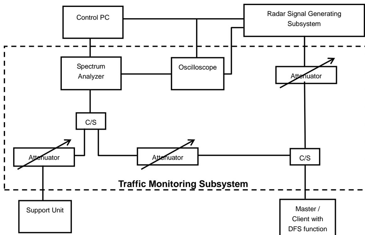
The test transmission will always be from the Master Device to the Client Device. While the Client device is set up to associate with the Master device and play the NTIA DFS MPEG file (6  $\frac{1}{2}$  Magic Hours) from Master device, the designated MPEG test file and instructions are located at:
