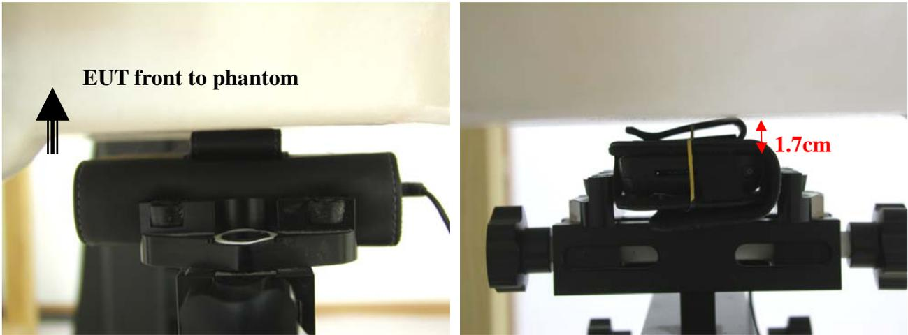
Fig.8 Body position with holster & belt clip and EUT front to phantom (testing in GPRS Mode), distance between flat phantom and mobile phone is 1.7 cm
