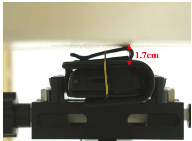
Fig.7 Body position with holster & belt clip and EUT back to phantom (testing in GPRS Mode) distance between flat phantom and mobile phone is 1.7 cm
