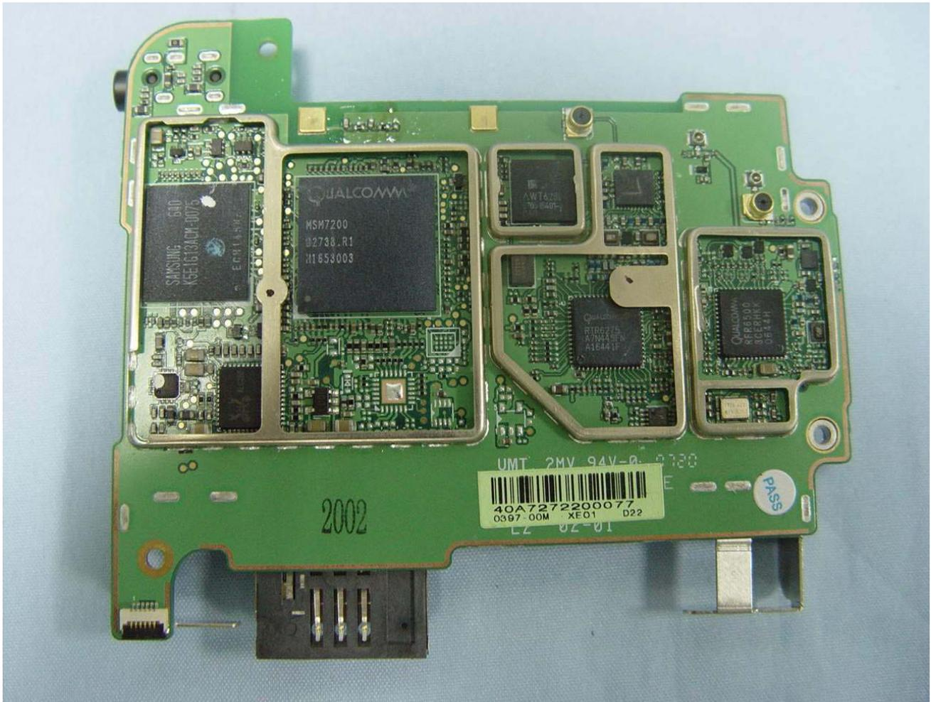
WWAN circuit block and antenna connectors
