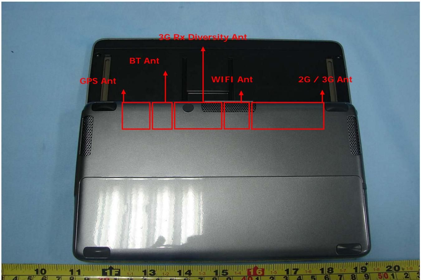
The exterior case of EUT relates to all of antennas positions
