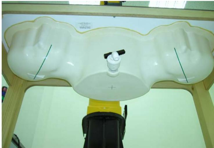
**Fig. 5.4 Bottom view of twin phantom**
