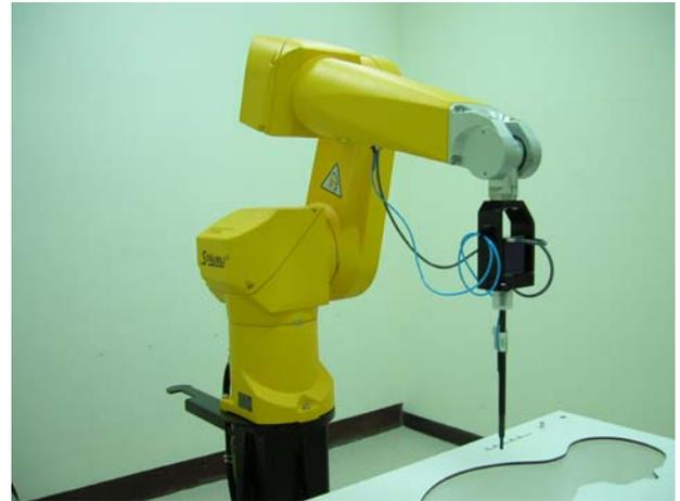
**Fig. 5.2 Probe setup on robot**
