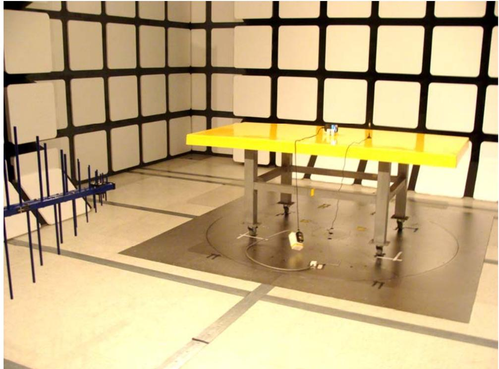
EUT with CDMA cellular 1xEV-DO Rev. A Link and BT Link Mode
