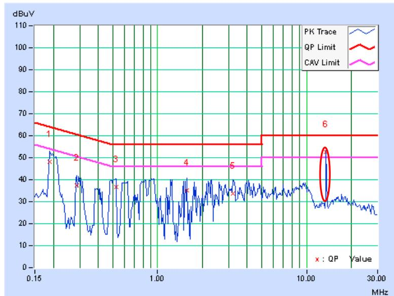
**Test with suitable dummy load**
