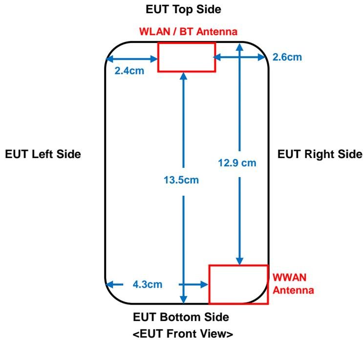
This device supports WiFi hotspot function, so body SAR was tested under 1 cm for the surfaces / slide edges where a transmitting antenna is within 2.5 cm from the edge. Since the SAR is required for antenna located within 2.5 cm from edge, SAR testing for each antenna is listed as below.
