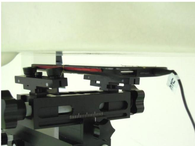
**Front Face of DUT with 1 cm Gap
