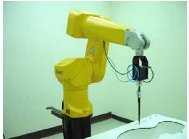
Fig. 5.2 Probe setup on robot
