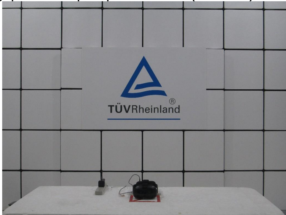
Photograph 9: Test Setup for Spurious Emissions (Front View 1)
