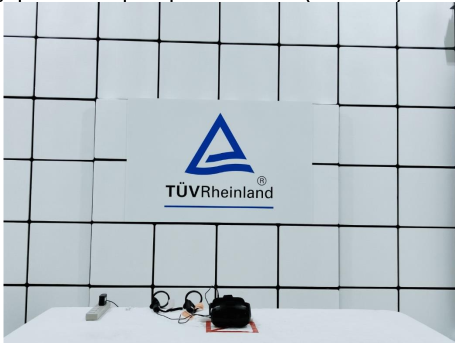
Photograph 1: Test Setup for Spurious Emissions (Front View 1)
