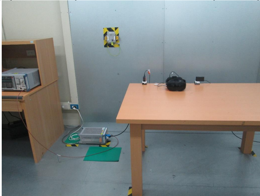
Photograph 12: Test Setup for Mains Conducted Emissions (Front View)
