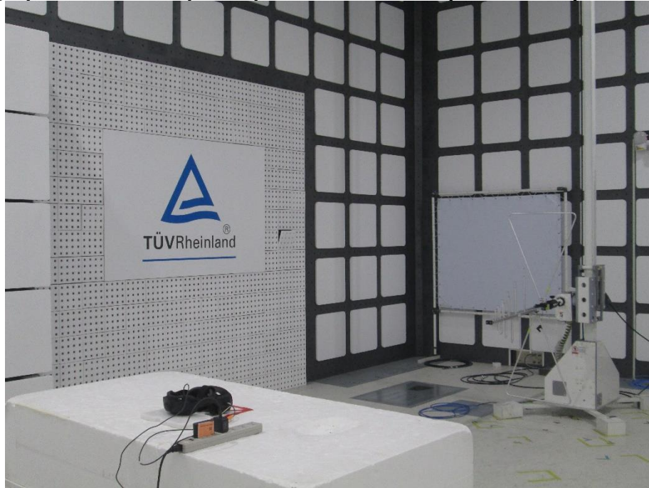
Photograph 11: Test Setup for Spurious Emissions (Back View 2)
