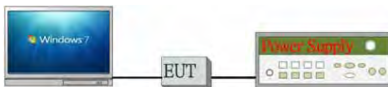
Fig. 2-2 Conducted (Antenna Port) Configuration
