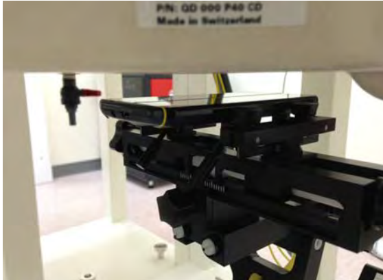
Fig.7 EUT front to flat phantom
