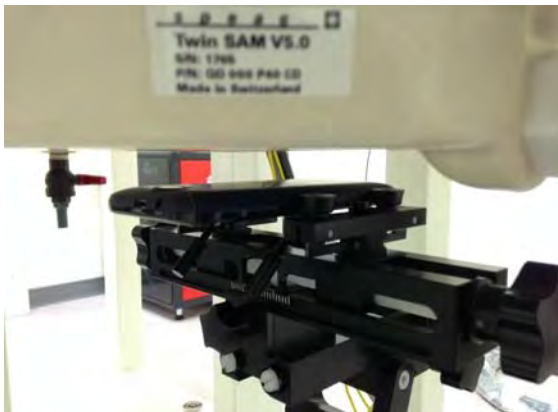
Fig.8 EUT back to flat phantom
