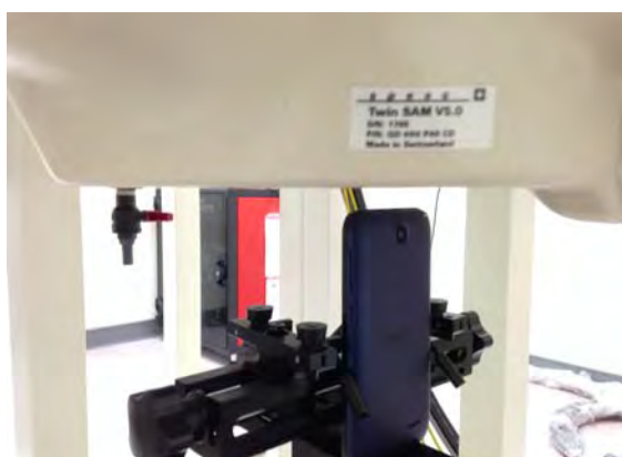
Fig.11 EUT top to flat phantom
