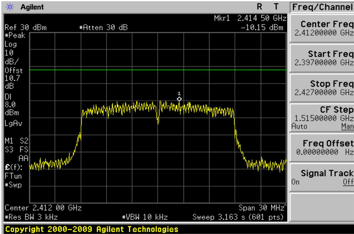
Power Spectral Density Test Plot (CH-Mid)
