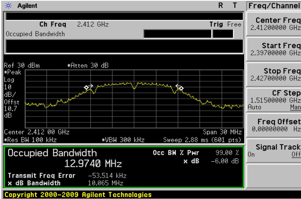
6dB Band Width Test Data CH-Mid
