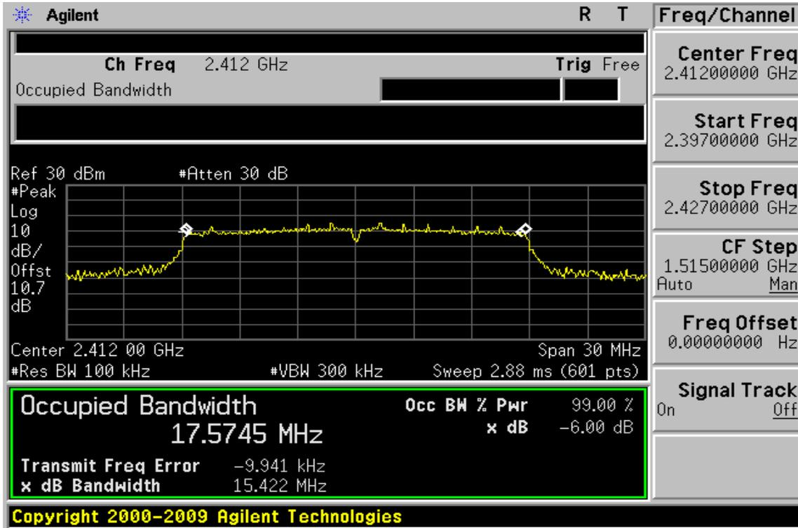
6dB Band Width Test Data CH-Mid
