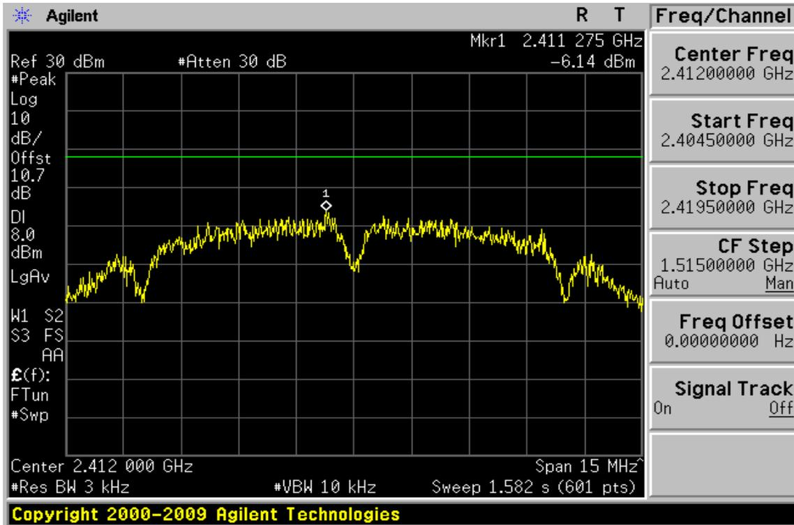
Power Spectral Density Test Plot (CH-Mid)
