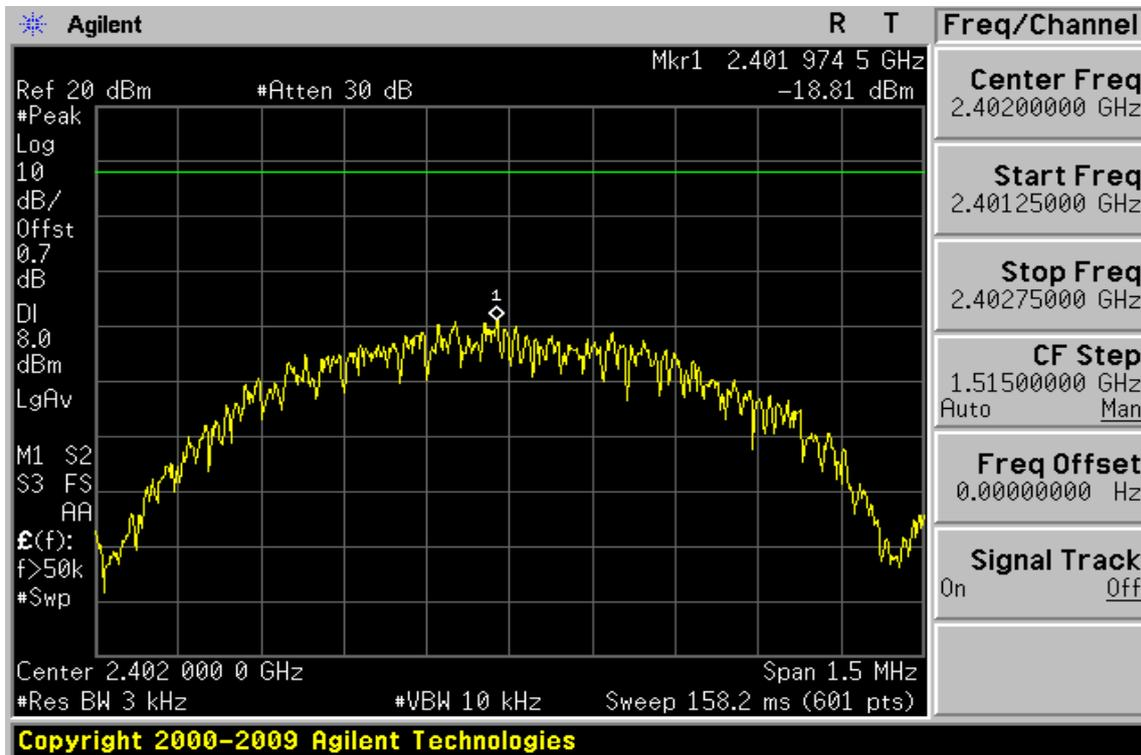
**Power Spectral Density Test Plot (CH-Mid)**
