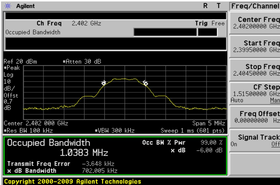
**6dB Band Width Test Data CH-Mid**
