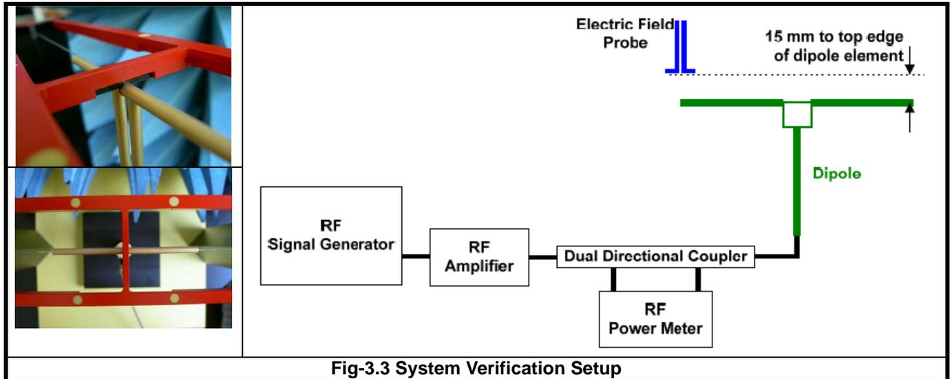
The validation dipole is placed beneath the center of arch phantom. The power meter measures the forward power at the location of the system check dipole connector. The signal generator is adjusted for the desired forward power, 100 mW (20 dBm) at the dipole connector and the RF power meter is read at that level. After connecting the cable to the dipole, the signal generator is readjusted for the same reading at RF power meter.
