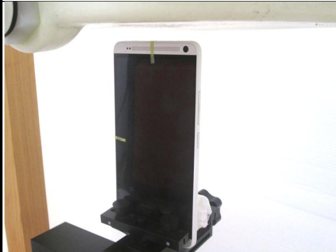
Top Side of EUT with 1.0 cm Gap
