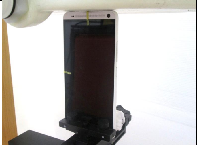
Top Side of EUT with 0 cm Gap
