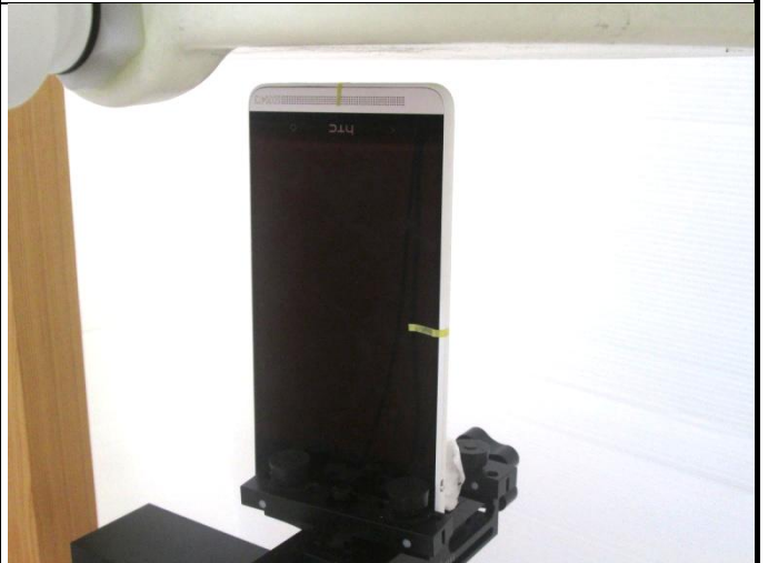
Bottom Side of EUT with 1.0 cm Gap
