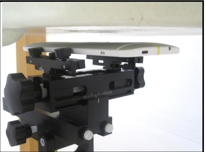
Rear Face of EUT with 1.0 cm Gap
