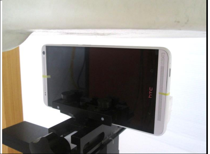
Right Side of EUT with 1.0 cm Gap
