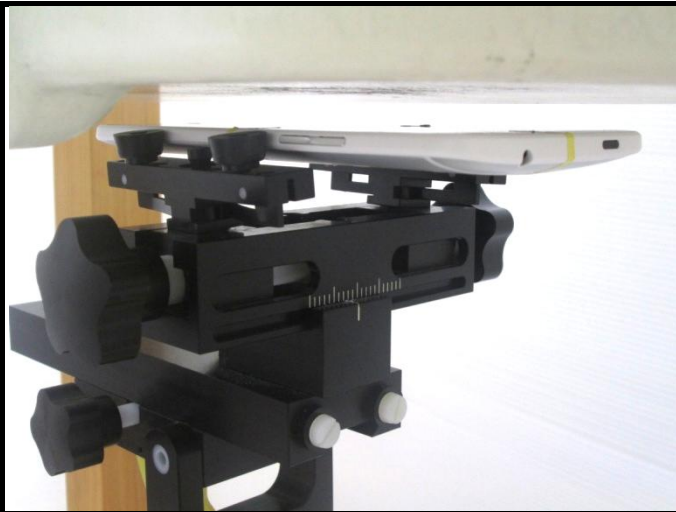
Front Face of EUT with 1.0 cm Gap
