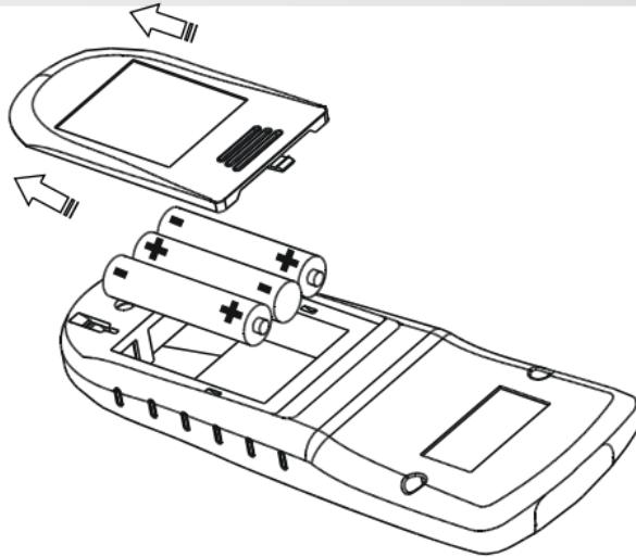
Insert the batteries in the battery compartment as indicated in figure and close the compartment.
