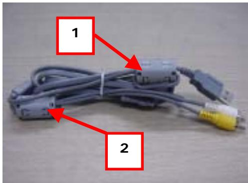
Ferrite Cores were inserted additionally.
