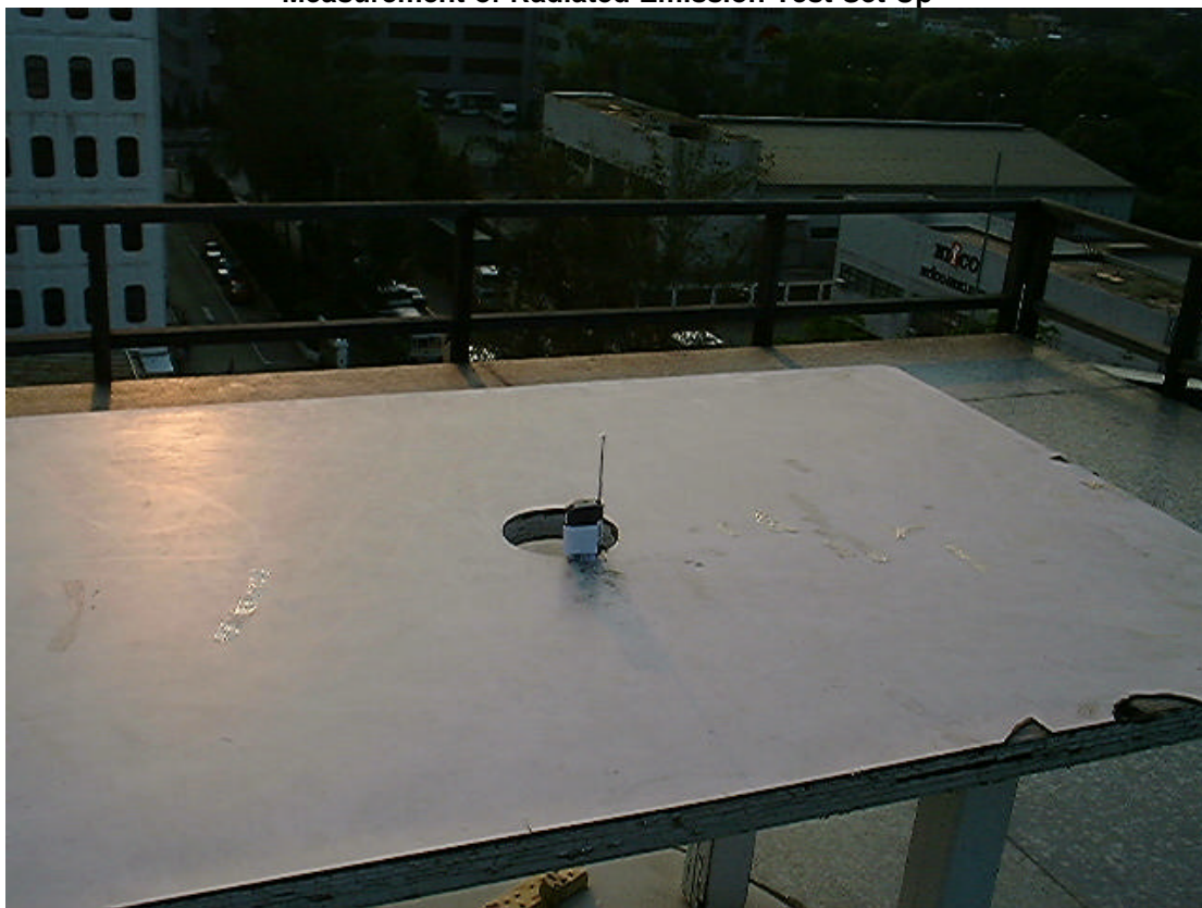
Measurement of Radiated Emission Test Set Up
