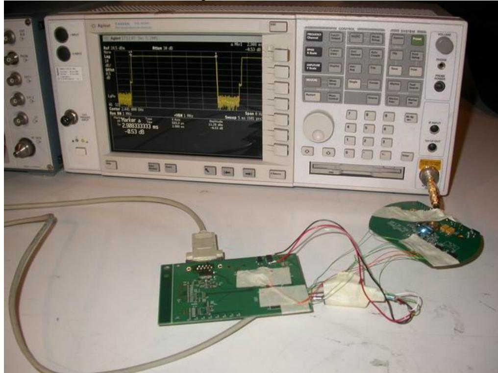
**POWERLINE CONDUCTED EMISSIONS MEASUREMENT SETUP**
