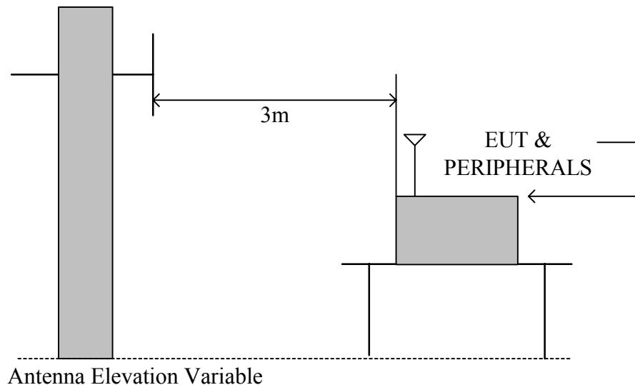
The diagram below shows the test setup that is utilized to make the measurements for emission above 1GHz.
