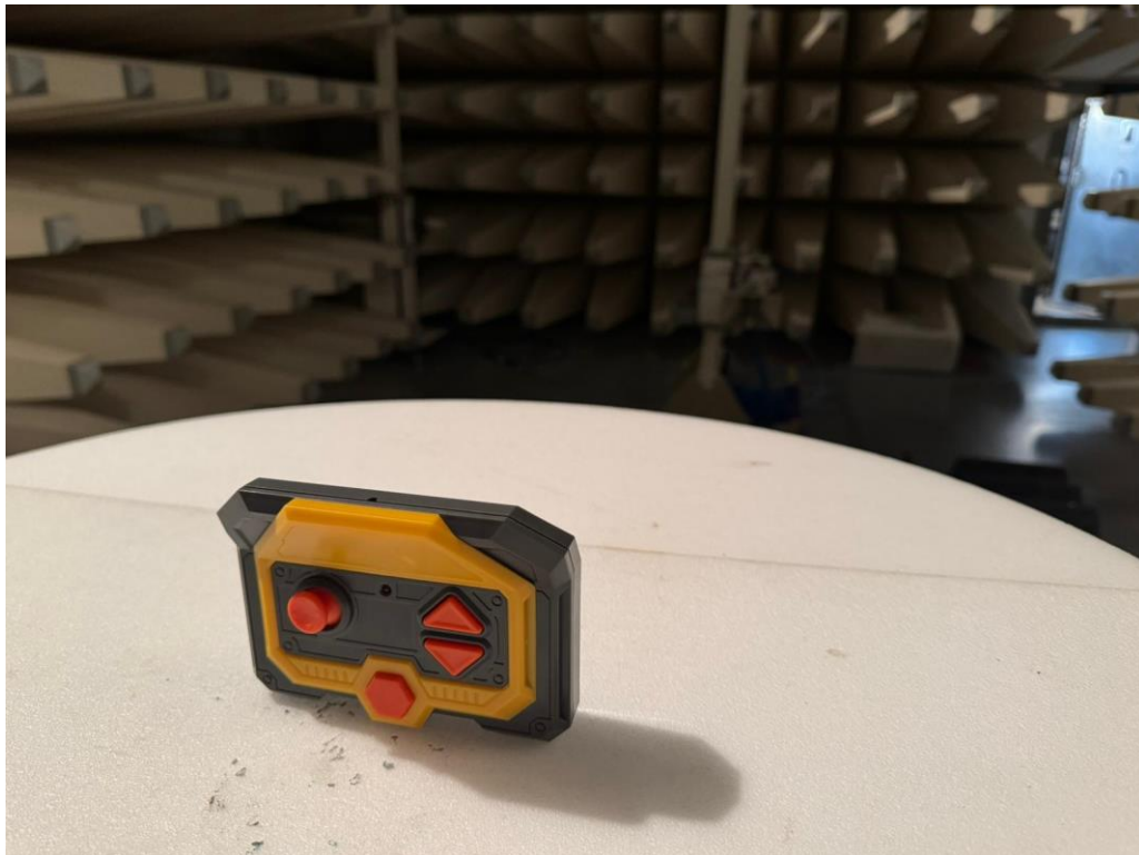
Set-up for Radiated Emission (1 GHz above)
