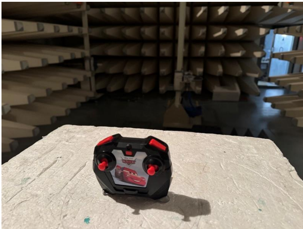
Set-up for Radiated Emission (1 GHz above)
