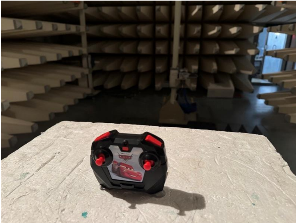
Set-up for Radiated Emission (1 GHz above)
