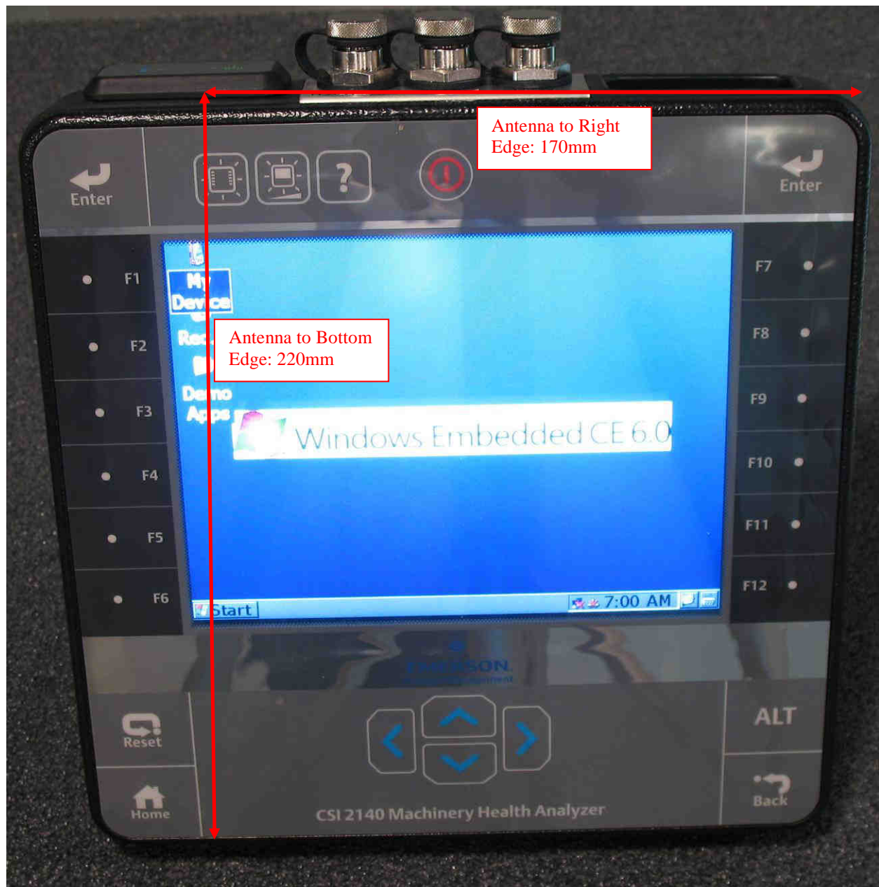
Figure 9: Antenna Spacing from Edges
