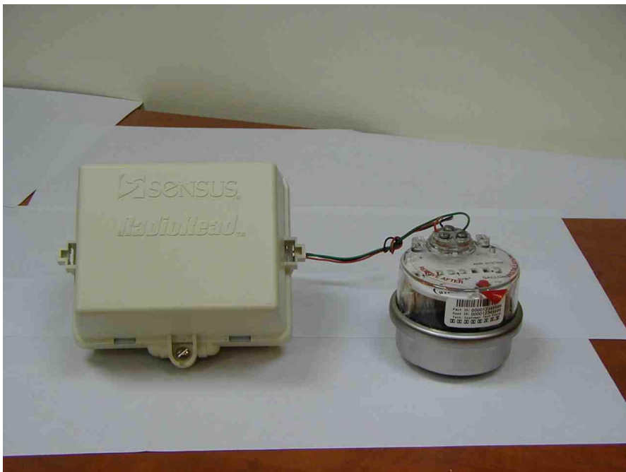
Figure 65 Transmitter Connected to Water Meter
