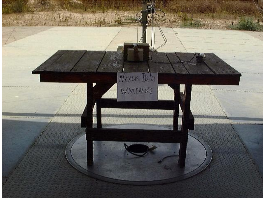
Figure 5. Spurious Radiated Emission Test. Front
