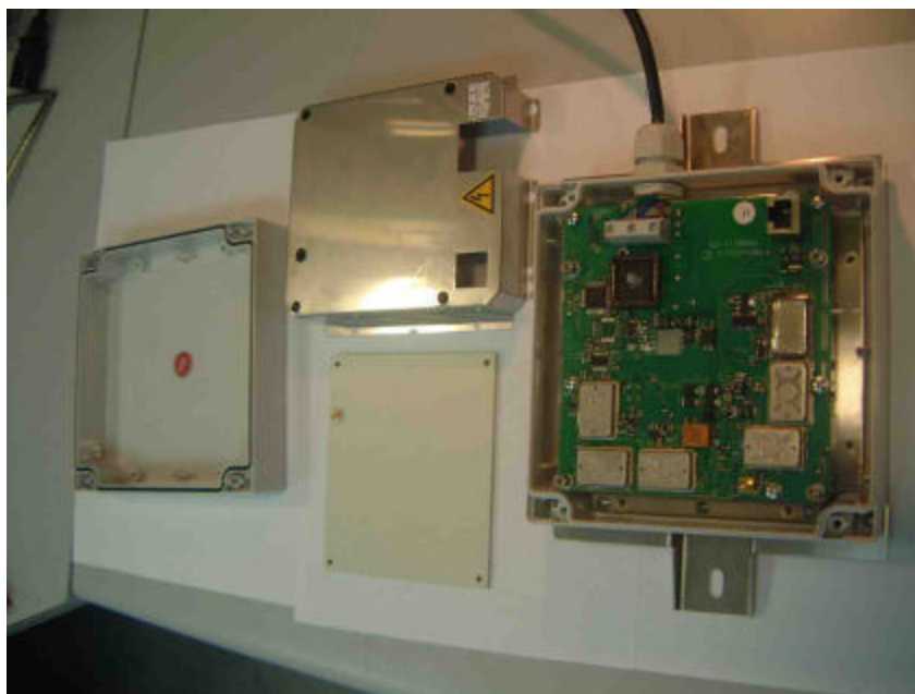
Figure 86 Printed Circuit Mounted in Housing/ E.U.T. Disassembled
