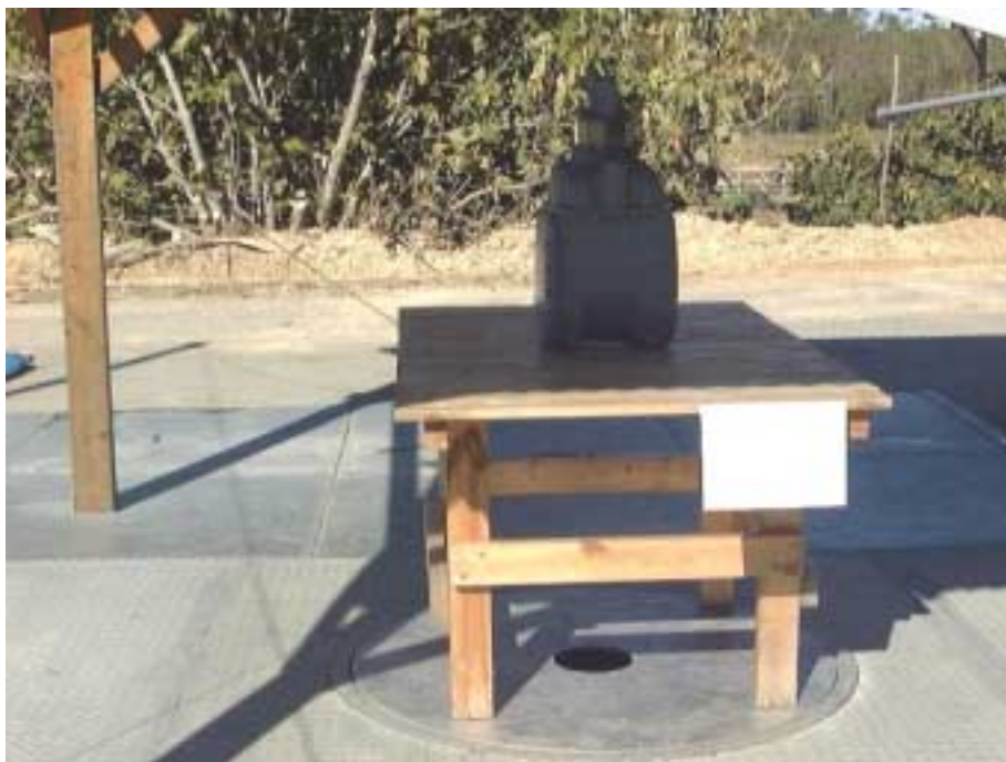
Figure 6. Radiated Emission Test. Side
