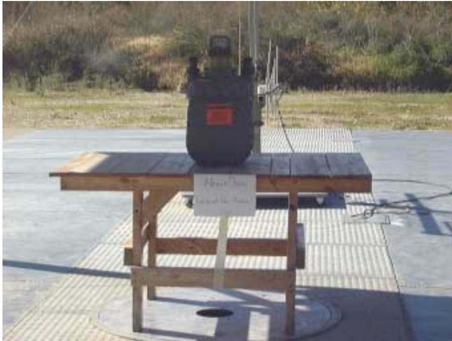
Figure 5. Radiated Emission Test. Front
