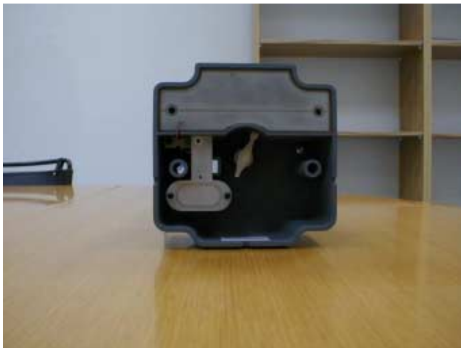
Figure 78 Printed Circuit Mounted in Housing
