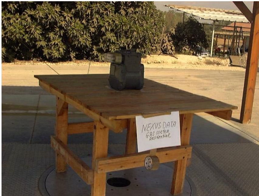
Figure 6. Radiated Emission Test. Side
