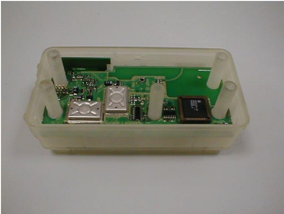
Figure 3 Printed Circuit Mounted in Housing
