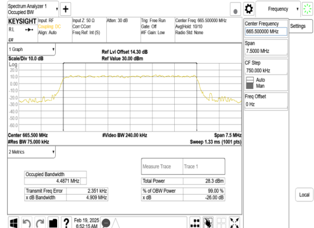
Band71_5MHz_DFT_s_OFDM_SCS15kHz_64QAM_RB25_0_CH133100
