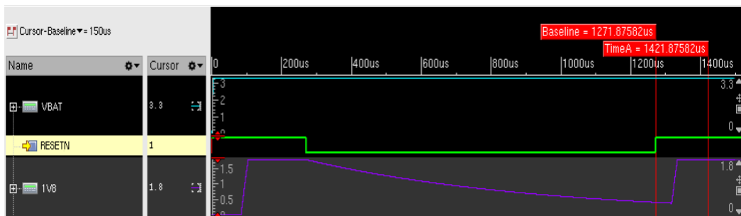
Figure 8. Typical Timing Diagram for Reset Sequence
