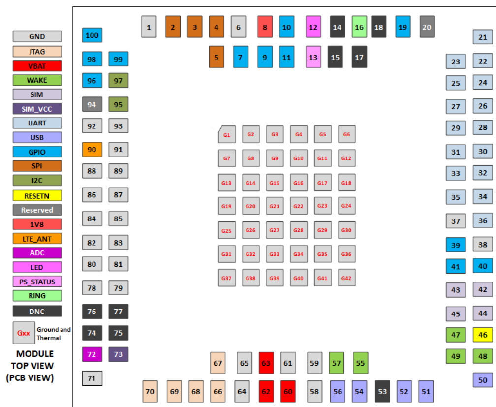
Figure 2. DLUS-WI01-NA Modules Pads Assignment
