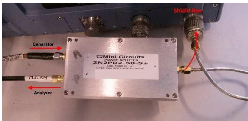
Figure 27. Configuration for Calibration and Screening
