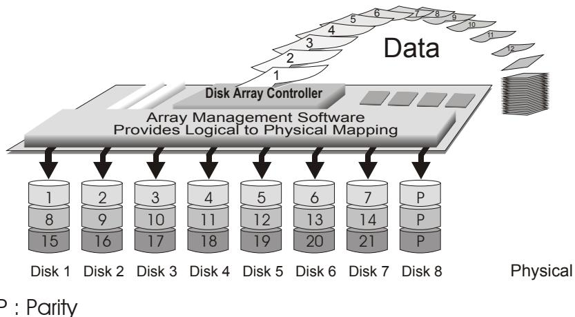
RAID Level 3 technology uses a dedicated parity disk to store redundant information about the data on several data disks. RAID Level 3 is an excellent choice for applications which require single stream I/O with a high data transfer rate.
