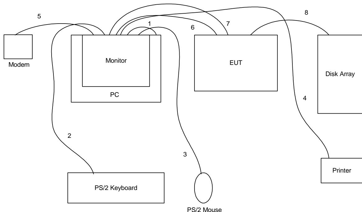
1. The I/O cable is connected from PC to the support unit 2.
