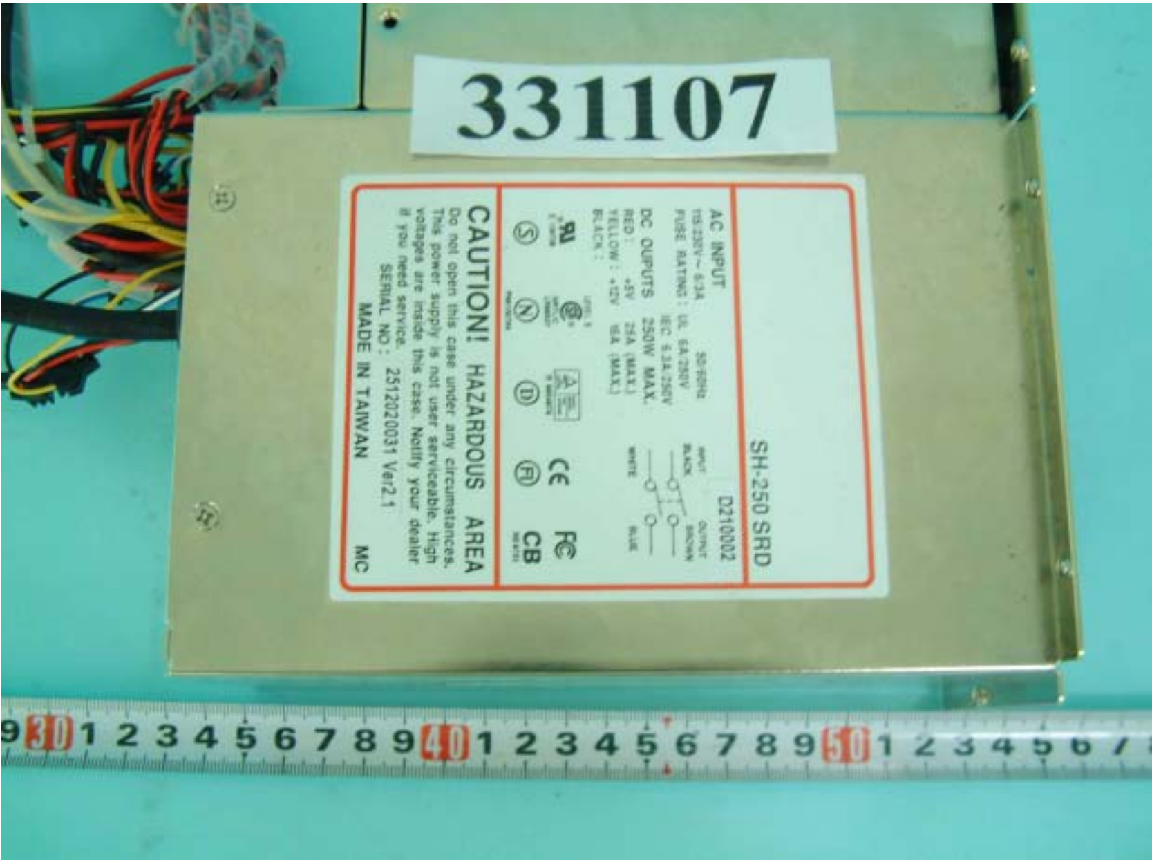
Front side of power
